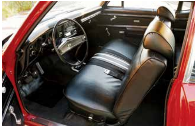
■ No bucket seats or even Astro ventilation here. The base 300 Deluxe Chevelles were equipped with bench seats like a taxi cab—Chevrolet even scrimped on the amount of foam in the seat cushion!—rubber floor mats, and vent windows.
