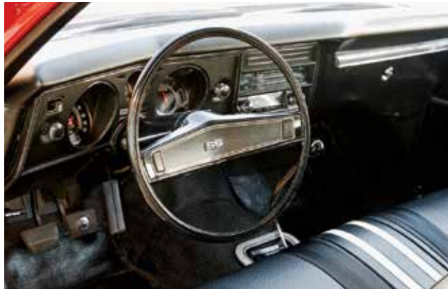
■ The instrumentation, too, is in keeping with the car’s base-level equipment. There’s no console on the floor either, but that’s a Hurst shifter coming out of the hole in the floor, likely added when the original owner swapped transmissions.
