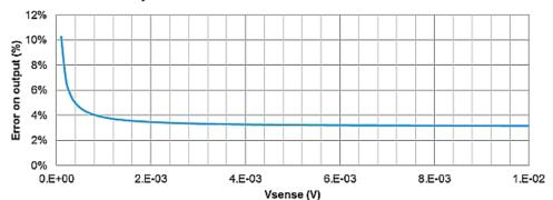
Figure 2: Total error assuming 1% resistances with Rshunt 1%
