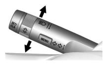
D: Push the turn signal lever away from you and release, to turn the high beams on.
