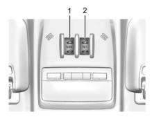
If equipped, the sunroof only operates when the ignition is on or when Retained Accessory Power (RAP) is active. See Retained Accessory Power (RAP) \( \Display 181. \)
