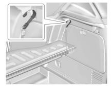
Fold the load floor. Place the hook from the load floor inside the hook on the side trim.
