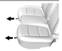
Pull the strap on the front edge of the rear seat cushion to release the cushion. Tilt the seat cushion forward toward the front of the vehicle.
