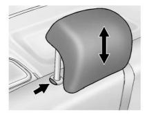
To lower the head restraint, press the button, located on the top of the seatback, and push the head restraint down.
