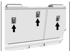
The top tether anchors are on the back of the rear seatbacks. Be sure to use an anchor located directly behind the seating position where the child restraint will be placed.
