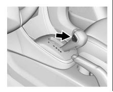
DSC allows you to shift an automatic transmission similar to a manual transmission.
