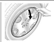
Remove the wheel cover, if the vehicle has one, to reach the wheel bolts.
