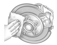
Remove any rust or dirt from the wheel bolts, mounting surfaces, and spare wheel. 11. Place the spare tire on the wheel-mounting surface.
