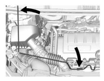
Lift the hood and release the hood prop rod from its retainer, in the front of the engine compartment. Securely insert the rod end into the slot marked with an arrow, on the underside of the hood.
