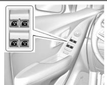
Power windows work when the ignition is on, in ACC/ACCESSORY, or when Retained Accessory Power (RAP) is active. See Retained Accessory Power (RAP)
