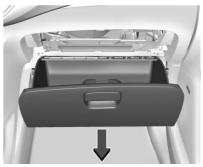
2. Push in both sides of the glove box and pull to remove.
