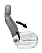
3. Lift the lever fully and fold the seatback forward.
