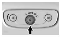
The exterior lamp control is on the instrument panel to the left of the steering column.
