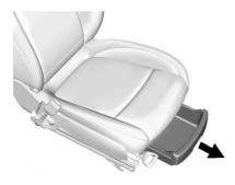
If equipped, there is storage under the front passenger seat. Lift the end of the tray up and pull it forward to open. Push it in toward the seat to close.
