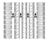
Treadwear indicators are one way to tell when it is time for new tires. Treadwear indicators appear when the tires have only 1.6 mm (1/16 in) or less of tread remaining. See *Tire Inspection* ⇔ 267 and *Tire Rotation* ⇔ 268.
