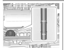
When the engine is hot, the level should be at the hot MAX level. When the engine is cold, the fluid level should be between MIN and MAX on the dipstick.
