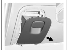
The instrument panel fuse block is on the underside of the driver side instrument panel. To access the fuses, remove the storage compartment. To remove the storage compartment, open the compartment and pull it out.
