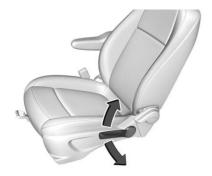
If available, move the lever up or down to manually raise or lower the seat.
