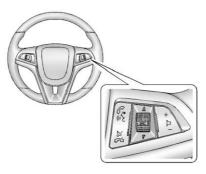
Some audio steering wheel controls could differ depending on the vehicle's options. Some audio controls can be adjusted at the steering wheel.
