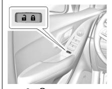
Press or to lock or unlock the doors, the liftgate, and if equipped, the locking fuel door.
