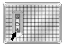
The rear dome lamp controls are in the headliner above the rear seats.
