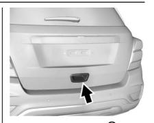
To open the liftgate, press and on the door lock switch or on the Remote Keyless Entry (RKE) transmitter to unlock all doors, then use the touch pad on the liftgate.
