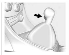
R (Reverse): To engage R (Reverse), with the vehicle stationary, pull up on the button on the shift lever and engage the gear. If the gear does not engage, set the lever in Neutral, release the clutch pedal, and apply it again; then repeat gear selection.
