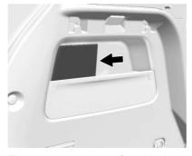
The rear compartment fuse block is behind a cover on the driver side of the rear compartment. To access the fuses, remove the cover.
