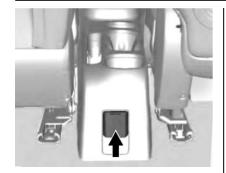
An indicator light on the outlet turns on to show it is in use. The light comes on when the ignition is on and equipment requiring less than 150 watts is plugged into the outlet, and no system fault is detected.
