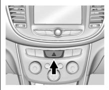
\(\textcal{\textcal{\textcal{\textcal{L}}}}\): Press to make the front and rear turn signal lamps flash on and off. This warns others that you are having trouble. Press again to turn the flashers off.
