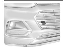
If equipped, carefully open the cover by using the small notch that conceals the tow eye socket.
