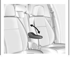
There may be an armrest on the inboard side of the driver seat. To raise or lower the armrest, push up or pull down on the armrest.
