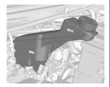
With the vehicle in P (Park) on a level surface, the brake fluid level should be between the minimum and maximum marks on the brake fluid reservoir.
