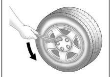
Turn the wheel wrench counterclockwise to loosen the wheel nuts. Do not remove them yet.
