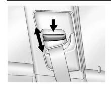
To move the shoulder belt height adjuster down, push down on the release button and move the height adjuster to the desired position. You can move the height adjuster up by pushing up on the shoulder belt guide.
