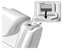
Reach under the belt and pull the lever on top of the seatback to unlock the seatback.
