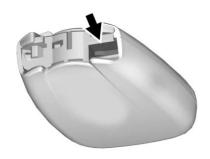
Separate the two halves of the transmitter using a flat tool inserted into the area near the key slot.
