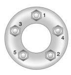
Tighten the wheel nuts firmly with the wheel wrench in a crisscross sequence, as shown.
