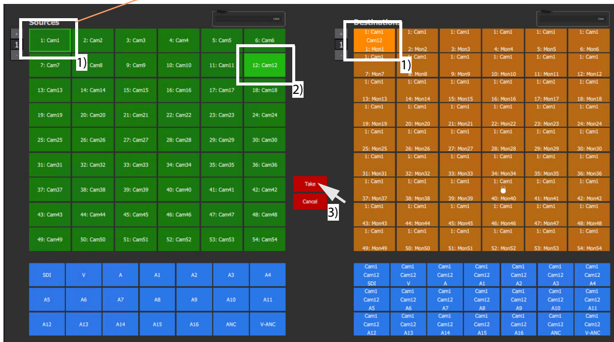
Fig. 6-21: Making a Simple Route
