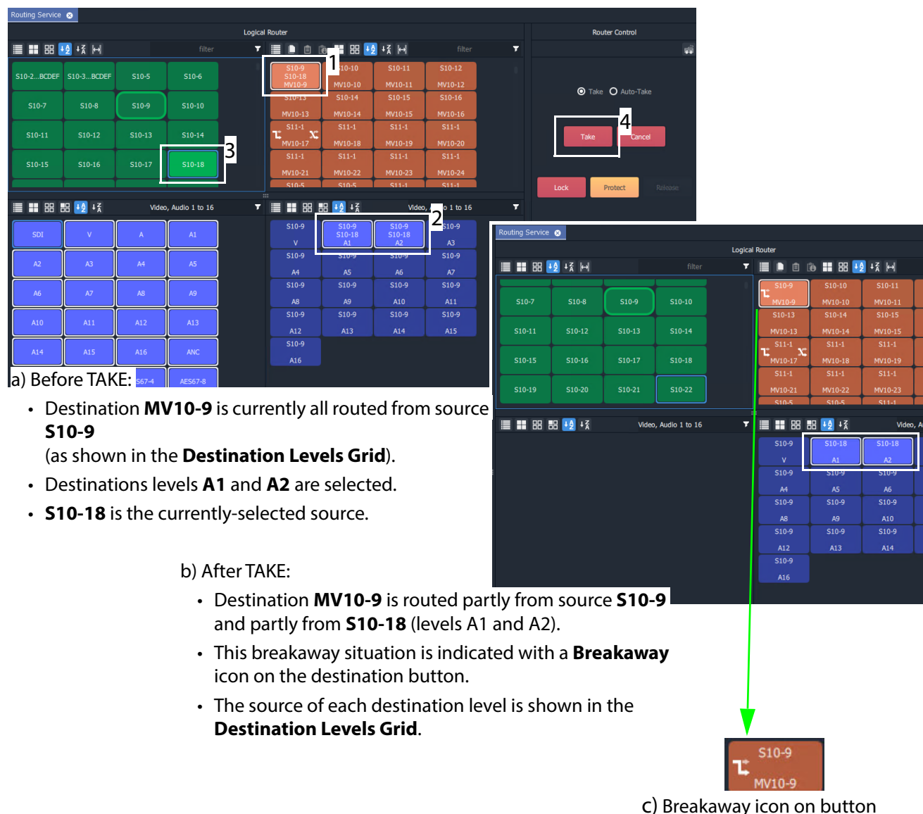
Fig. 5-33: Breakaway Example: a) Before TAKE; b) After TAKE; c) Breakaway Icon on Button.
