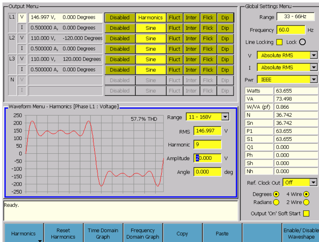
Figure 4-9. Harmonics with time domain graph
