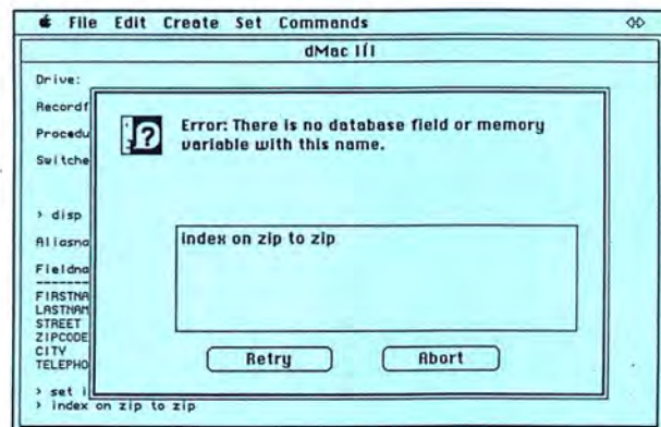
Fig. 2: A dialog box provides detailed information about the nature of syntax errors in dMac III programs. However, it does not tell the user in which program the offending line was found.
