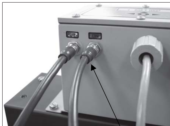
Figure 3 Connect Transducer Cables
