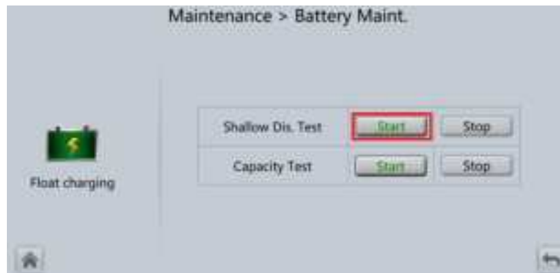
Figure 5-13 Starting a shallow discharge test
