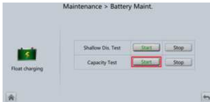
Figure 5-14 Starting a capacity test
