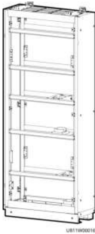
Figure 2-15 Fire extinguishing cabinet
