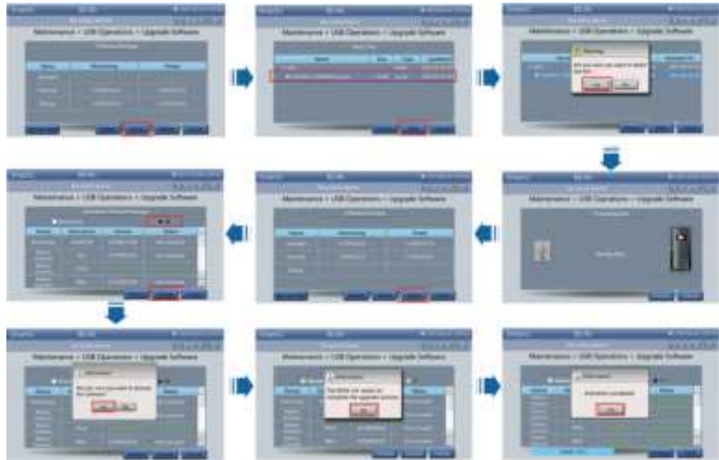
Figure 10-5 Uploading and activating the software (the BCB of a single battery cabinet is OFF)
