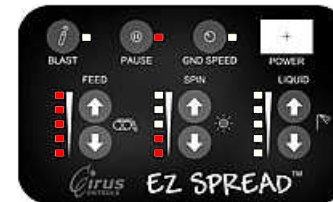
Pause LED On (spreading paused) Feed LED=10, Spin=4, Liq=0
