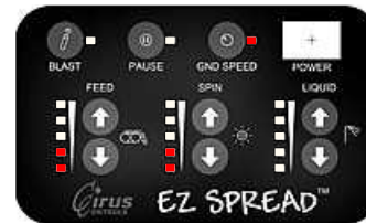
GND LED On constant, spread normal Ground speed oriented.
