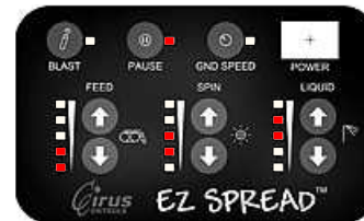
Pause LED On (spreading paused) Feed LED=2, Spin=4, Liq=6
