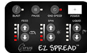
If feed, spin, or aux LED's are flashing, an open or shorted electric circuit is detected and output for that channel is turned off.
