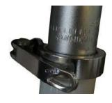
If the safety line on the seat tube is visible (as seen in the picture to the left), then lower the seat until the safety line is NOT visible. Once the safety line is NOT visible, then lock your seat into the desired height and make sure the seat is fastened and secured properly.
