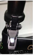
Front Folding Stem: On the bar that connects the handlebar to the front fork, locate the locking lever. Once located, lift the lever and pull down towards floor. Then pull down the safety locking lever and then at the same time push down the stem until it is fully folded.
