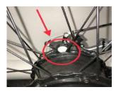
If you feel that your brakes are too tight, turn the silver knob clockwise (clockwise is to the right) and now try to see how the braking of the bike wheel feels. Turning the silver disc clockwise will loosen the brakes, as where turning the silver knob counter-clockwise will tighten the brakes.
