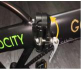
Frame: First locate the locking lever in the middle of the bike frame. Then pull the lever towards rear of bike. Then push lever upwards and this will fold the bike frame.
