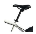
Open the release handle found on the frame of the bike. Then insert the seat tube into the frame. (as seen in the picture to the left) Adjust the saddle to find the right height for riding your GoPowerBike.
