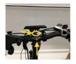
The Handlebar comes folded. Lock the stem into place using the lock levers.
