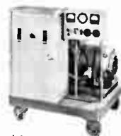
Portable, caster-mounted 400 cycle installation for production test equipment.
