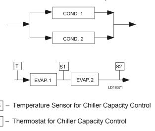
FIGURE 2 - SERIES EVAPORATORS PARALLEL CONDENSERS
