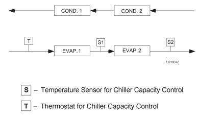
FIGURE 3 - SERIES EVAPORATORS SERIES-COUNTER FLOW CONDENSERS
