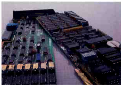
Expansion boards let you add memory and extra functions inside, not out.
