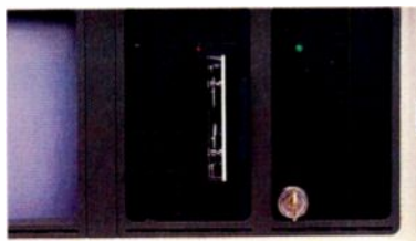
Two data protection features from COMPAQ: an internal fixed disk back-up system that stores data on tape cartridges, and a security lock for locking keyboard access to your system on or off.
