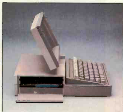
Photo 4: Behind the door on the Pro-Lite's left are the two slots for plugging in options: an RS-232C interface, 300-bps modem, external color monitor interface, or Solid State Software drawer.
