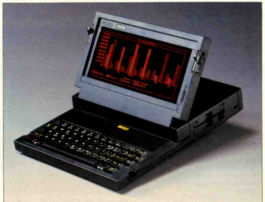
Photo 1: The GRiDCase III with the gas-plasma display. GRiDPlot, GRiD's proprietary graphics package, is shown on the screen.
