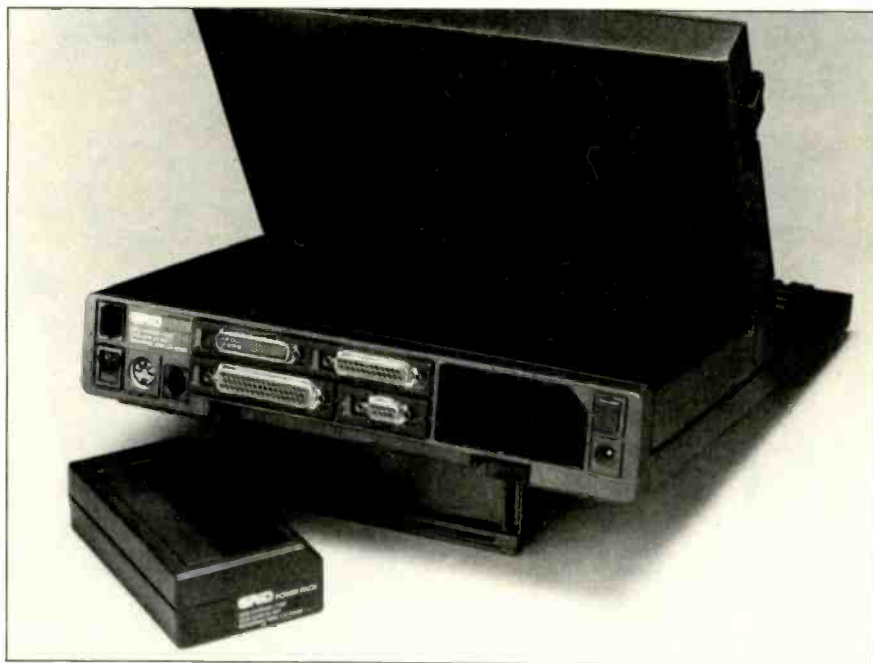
Photo 3: The GRiDCase back panel (left to right): the DIN connector for the IBM PC keyboard or 10-key keypad, the built-in 300/1200-bps modem (Hayes Smartmodem-compatible), RS-232C serial interface, external bus connector for external GRiD peripherals and access to the IBM PC expansion chassis, Centronics parallel interface, color (RGB) video-out for external monitors, built-in rechargeable/exchangeable battery pack.
