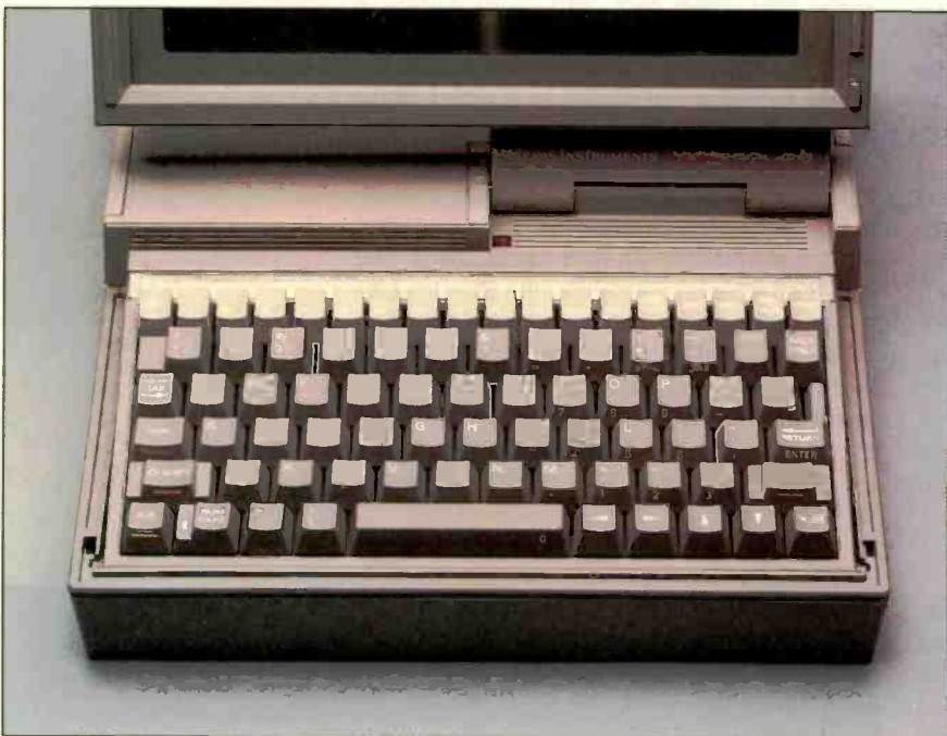
Photo 2: The Pro-Lite keyboard. Note the embedded numeric keypad, the 12 programmable function keys, and the overlay slot for labeling the function keys.
