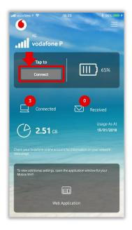
If there are issues in the connection action, namely an error message being shown to the user, it's also possible to perform this action on the mobile Wi-Fi router configuration landing page. The user can access it by pressing the "Web Application" button in the Mobile Wi-Fi Monitor app or opening a browser and accessing the URL <a href="http://vodafonemobile.wifi">http://vodafonemobile.wifi</a>
