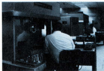
Fully automatic Gardner Denver machine wrapping
