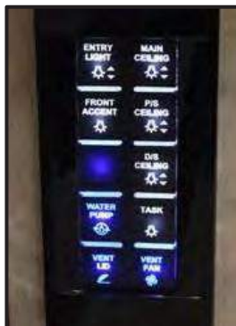
Figure 13-6: Water Pump Switch
