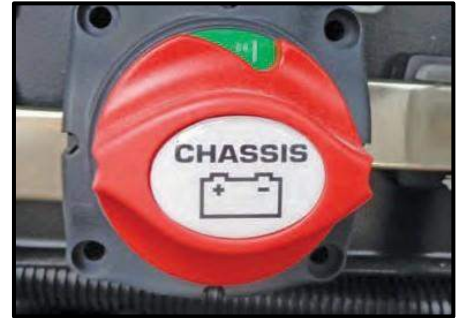
Figure 9-5: Engine Battery Disconnect Panel Switch
