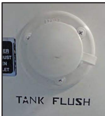
Figure 13-15: No Fuss Flush Connection
