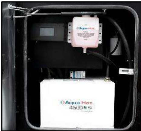
Figure 4-2: Aqua-Hot Surge Tank
