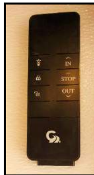
Figure 14-4: Awning Remote (located in the front cargo bay)
