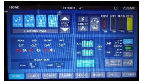
Figure 3-2: Home Screen for the Spyder Controls System
