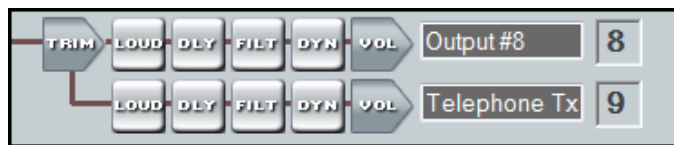
Figure 38. Telephone Tx Signal Path
