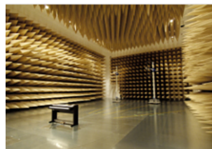
An anechoic chamber used for electromagnetic wave measurement
