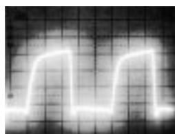
Signal Waveform (20ns/div / 1V/div)
