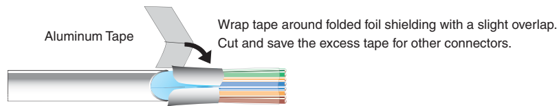
Figure 7. Wrapping the Shielded Tape
