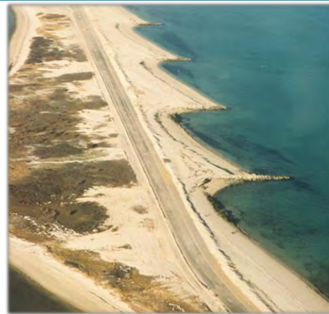
Photograph 2.11. Barrier beach with partial constraint to landward movement. Since it hasn't experienced a major storm in more than 10 years, dense beach grass and shrubs on this barrier beach are able to grow on the back side. The dunes on the seaward and landward side of the road can still erode and supply sediment to the beach in a storm event and perform all other dune functions. The function of the dune under the road has been diminished. However, in a large storm event, the pavement does break up and the dune can provide more function. Photograph courtesy of Jim Mahala, MassDEP.
