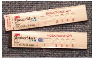
$3M^{TM}$  Monitor Mark  $^{TM}$  Time Temperature Indicators add an important temperature exposure measure that extends beyond your plant to your customers' delivery dock.
