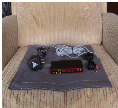
Figure 7. Oval Window (left) and Univox (right) induction listening systems.
