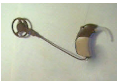
Figure 5. BTE cochlear implant: external processor and magnetic headpiece.
