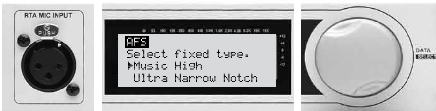
34A - Using the Data Wheel, choose the EQ notch filter width appropriate for your needs. Speech is a wide filter, Music Low is a narrow filter, Music Medium is a Very Narrow filter, and Music High is an Ultra Narrow filter (Music High Typical).
