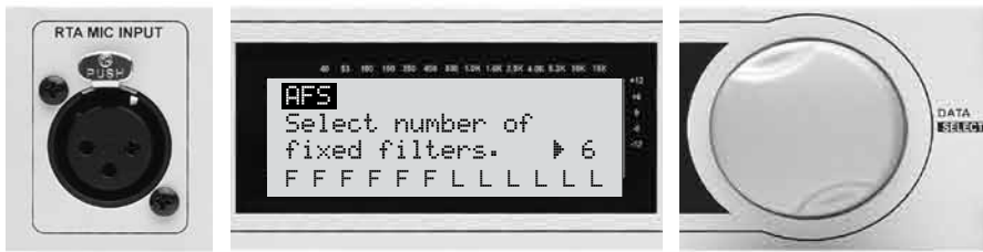
33A - Using the Data Wheel, choose the number of fixed filters to use with Advanced Feedback Suppression (AFS). These filters, once populated or FIXED, will stay at the set frequency and level. LIVE "L" filters will change as needed during a performance to eliminate further feedback.
