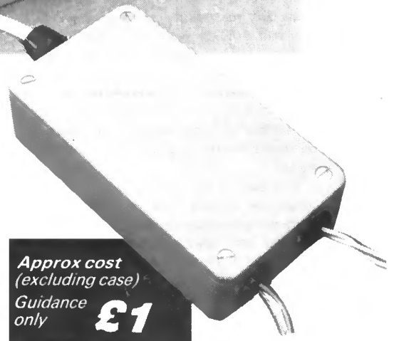
A completed "two string" lights protector. The resistors must be proud of the case-floor. Never remove the lid if the unit is still plugged into the MAINS and use a proper cable clamp for the mains lead..
