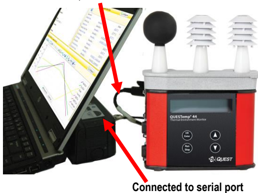
Figure 1-30: Communicating with the QT o 44/46 and DMS
