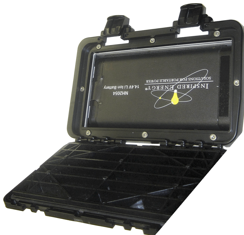
Figure 15. Slide Battery Door Clips Up To Open.
