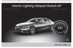
The interior lighting is activated for the duration of the delayed switch-off time when the key is removed from the ignition lock.
