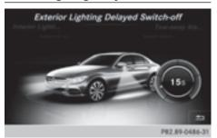
The locator illumination (surround lighting) is activated for the duration of the delayed switch-off time when the vehicle is unlocked using the remote control key.
