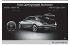
Activating the trunk lid opening height restriction allows you to avoid bumping the trunk lid on a low garage ceiling, for example.
