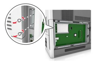
4 Remove the printer hard disk.
