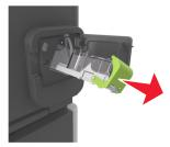
**3** Squeeze both sides of the empty staple case with your fingers, and then remove the staple case from the cartridge.
