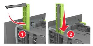
**d** Squeeze the length guide and slide it to the correct position for the size of the paper being loaded until it *clicks* into place.
