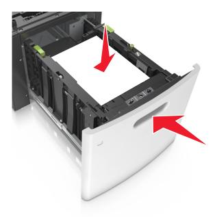
**6** From the printer control panel, set the paper size and type in the Paper menu to match the paper loaded in the tray.
