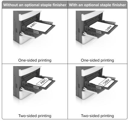
• If you are loading prepunched paper for use with the staple finisher, then make sure the holes on the long edge of the paper are on the right side of the tray.
