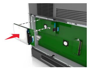
**c** Insert the plug of the printer hard disk interface cable into the receptacle of the ISP.
