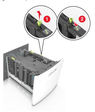
**b** Squeeze and slide the length guide to the position for A5 until it *clicks* into place.
