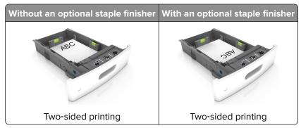
• If you are loading prepunched paper for use with the staple finisher, then make sure the holes on the long edge of the paper are on the right side of the tray.
