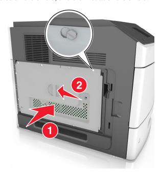
**6** Tighten the screws on the shield.
