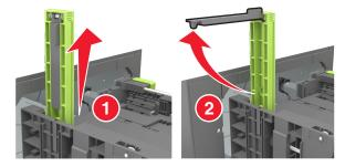
**d** Insert the A5 length guide into its designated slot.
