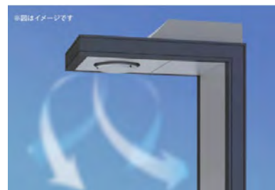
Air curtain creating dome-shaped cooling space
