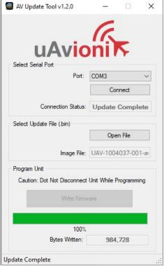
7. When the AV Update Tool displays "100%" and the lower status reads "Update Complete" the process is complete.
