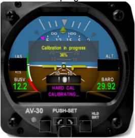
7. AV-30 will indicate "Calibration successfully completed Press DONE" Press the left button under "DONE" and the calibration will be complete. If an error is shown, repeat the calibration process.
