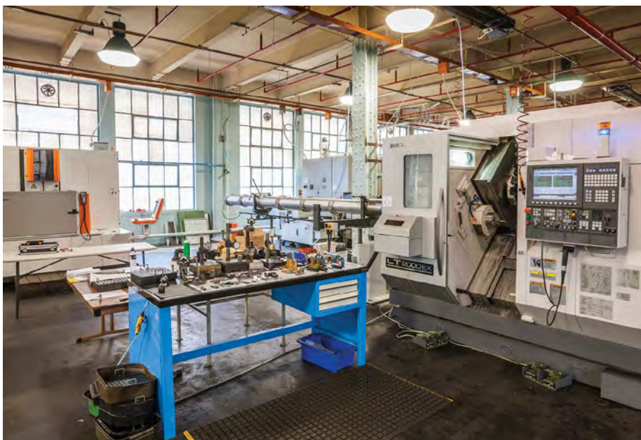
New Okuma LT2000EX mill turn lathe for EF88 bolt production. Image courtesy ThalesGroup Australia.
