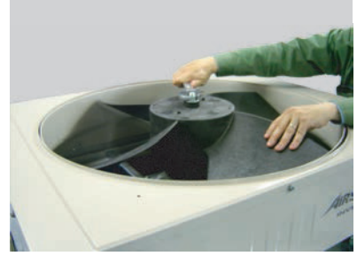
Remove the nut. Note the tightening torque at the installation. Tightening torque is from 15 to 20N·m.
