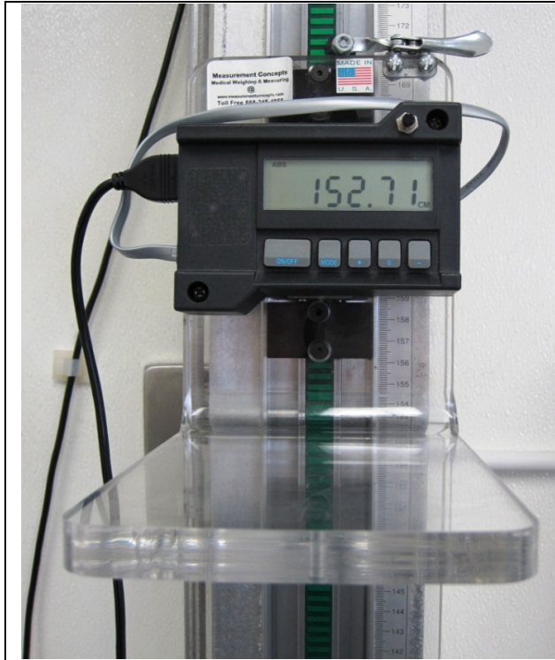
Exhibit 2-7. Stadiometer headpiece and digital measurement device
