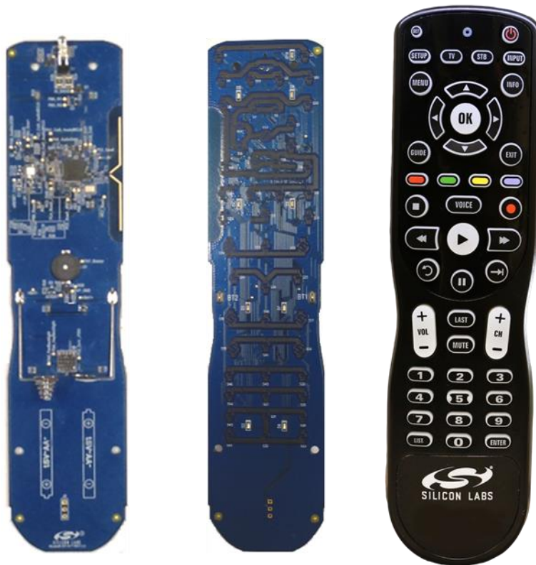
Figure 5: Silicon Labs ZigBee Remote Control Reference Design
