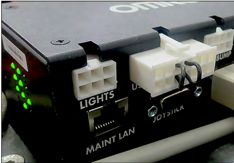
Figure 3-19. E-Stop Jumper on LD Platform Core
