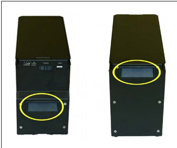
Figure 3-16. Battery Recesses, for Gripping
