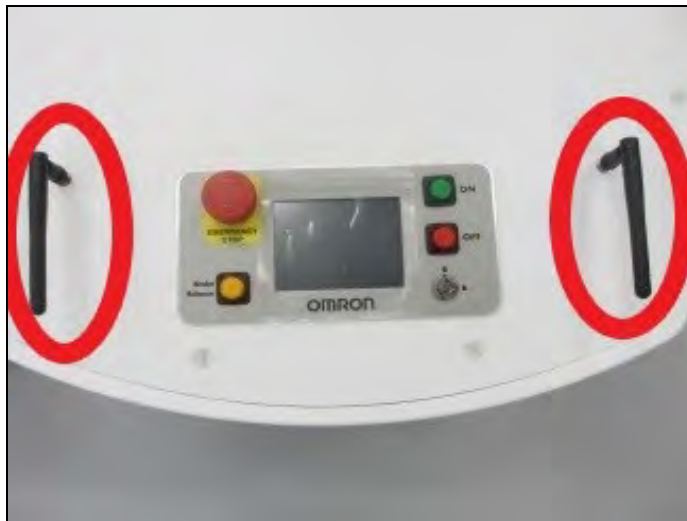
Figure 3-11. Robot Antennas Circled in Red
