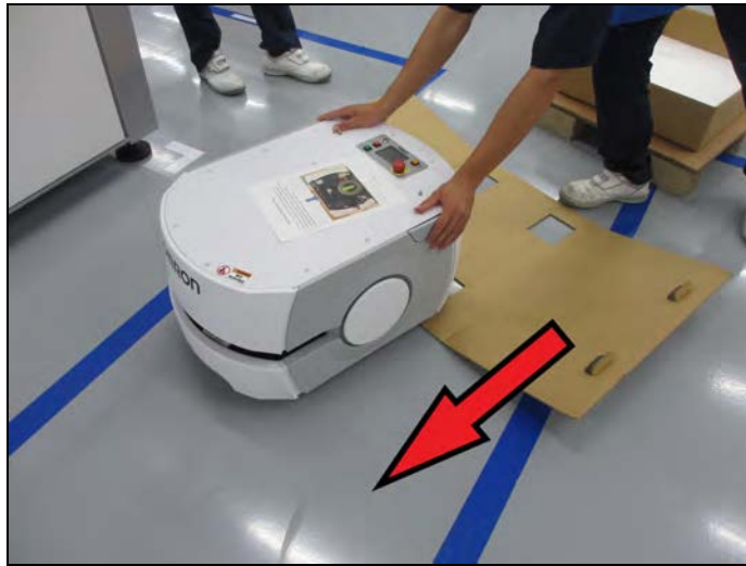
Figure 3-10. Robot Rolled onto the Floor
