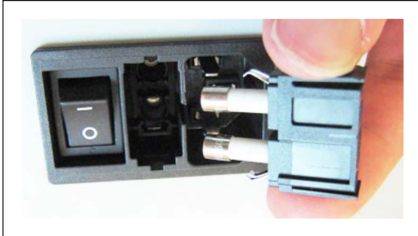
Figure 8-8. Docking Station Fuse
