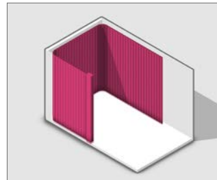
Fig. 4-5 One-door, right-locking (opening to the left)
