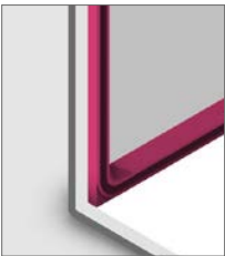
Fig. 4-30 top mounted (screwed)
