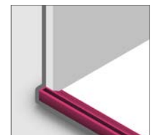
Fig. 4-9 front mounted (screwed)
