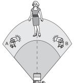
Divide the slave units into Groups A and B and change the flash ratio to obtain the desired lighting effect.
