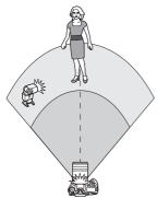
This is fully automatic wireless flash shooting with one external Speedlite and the built-in flash.
