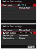
Normally, set this to [**E-TTL II**]. This enables autoexposure shooting with the built-in flash.
