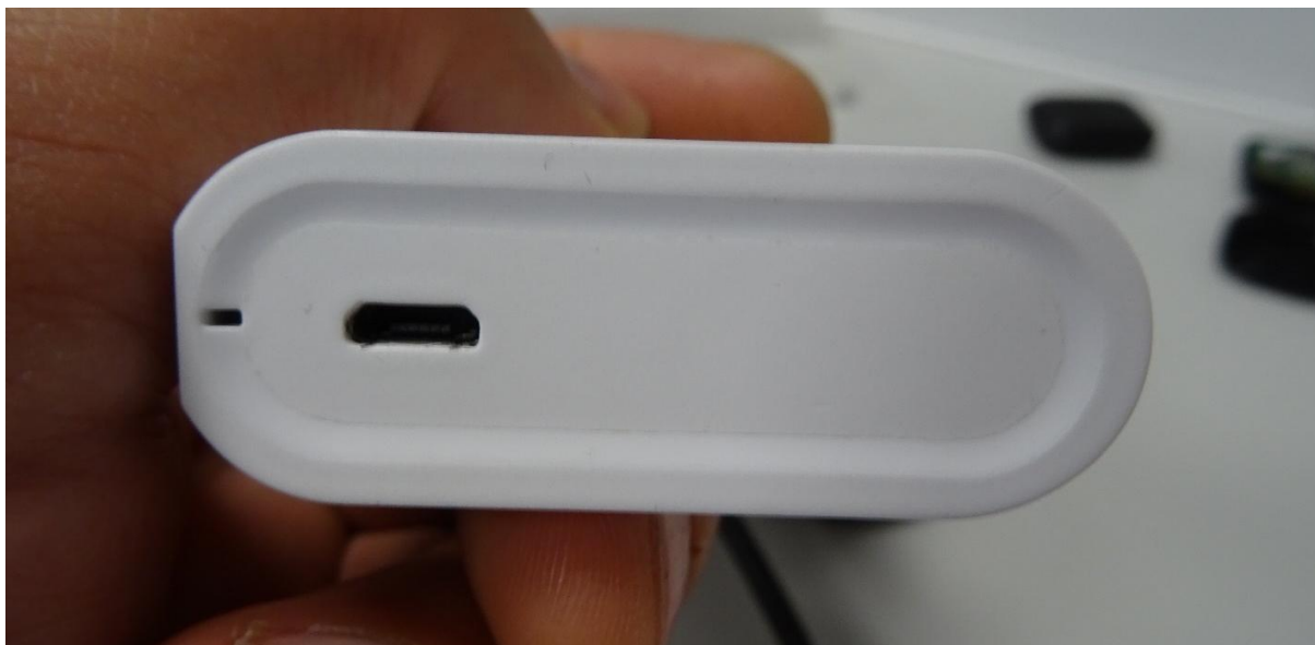
Picture 3: Power (USB) connection charger
