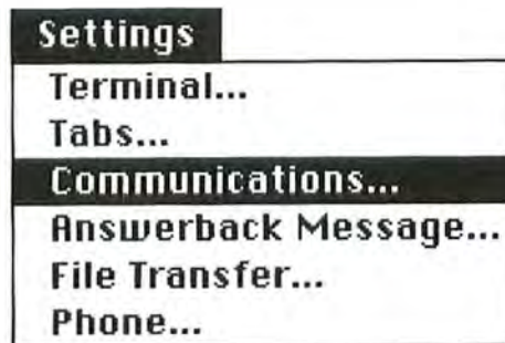
Figure 2 The Settings menu provides the terminal and file transfer features you'll need to communicate with other computers. Choosing a menu option gives you a dialog box with buttons or check boxes in which you select options, or windows in which you enter data such as phone numbers or answer-back messages.
