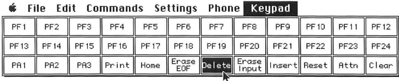
Figure 4 The Keypad is used when the Mac emulates an IBM model 3278 terminal. The 3278 terminal has several extra keys dedicated to special commands such as cursor movement and editing.
