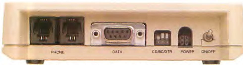
Sockets on the back of the Modem 1200 let you hook up to telephones and a telecommunications cable, and toggle switches enable you to configure various software and hardware combinations.
