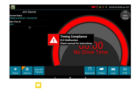
**WARNING:** If you are not able to immediately resolve the malfunction, you must begin keeping paper logs until the device is once again compliant. If your logs can no longer be accessed on the device, you must reconstruct your logs on paper for the current 24-hour period and the previous seven consecutive days.
