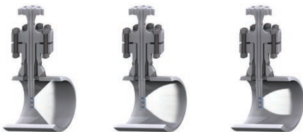
Figure 3: Attemperator overspray, proper spray, and underspray.
