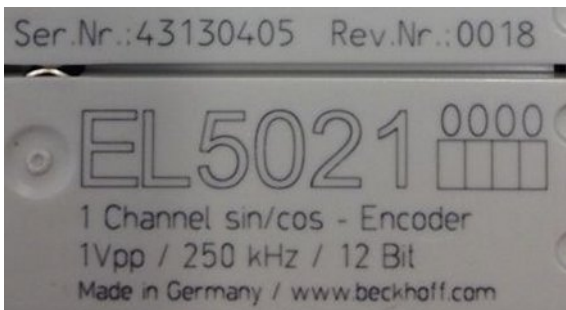
Fig. 27: EL5021 EL terminal, standard IP20 IO device with serial/ batch number and revision ID (since 2014/01)
