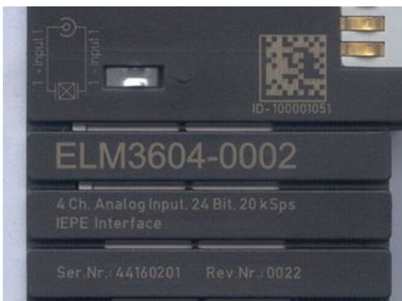
Fig. 34: ELM3604-0002 terminal with unique ID number (QR code) 100001051 and serial/ batch number 44160201
