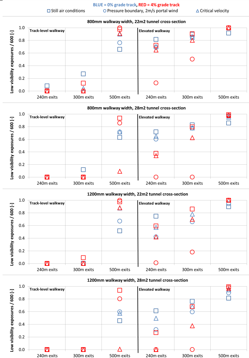
Figure 7. Number of agents exposed to less than 5m visibility for greater than 10 minutes. Values normalized by 600 (number of agents moving towards furthest exit).
