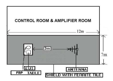
Note: The SPORTON 12m  $\times$  7m  $\times$  7m Fully Anechoic chamber is compliance with the sixteen points uniform field requirement as stated in IEC 61000-4-3 Section 6.2.
