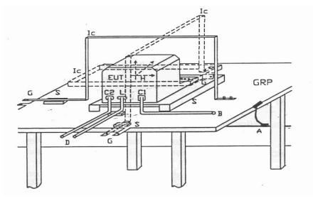
GRP: Ground plane C1: Power supply circuit
