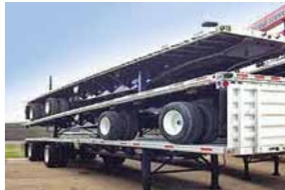
2003 Fontaine Combo Flatbed, (Qty: 10) Air Ride; 48 ft Length x 102 in Width; Aluminum Floor; 22.5 Tires; All Steel Wheels; Spread Tandem Axle; Combination Composition. (31516798-SHV-TRL-3b)
