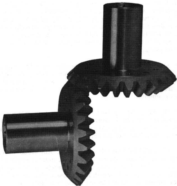
Figure 3-1. Bevel Gear - Showing Extreme Pitch Alignment
