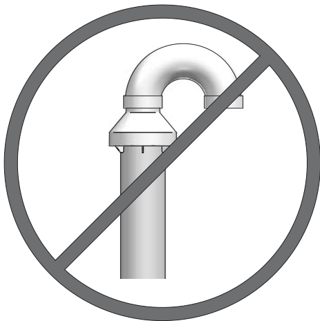
Figure 5-5 Do Not Install U-Bend to Rain Cap
