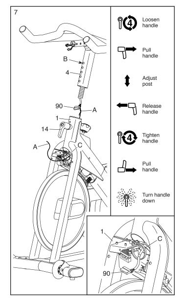
8. **See the inset drawing.** Connect the connector on the Handlebar Wire (90) to the connector on the Frame Wire (82).
