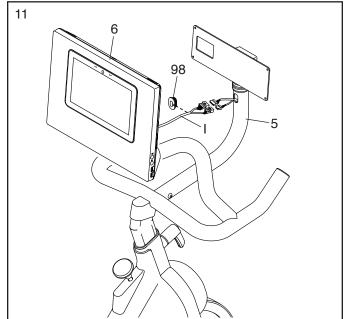
12. Connect the connectors on the Console Wire (I) to the connectors on the Mount Wire (91). Next, insert the connectors into the Console Mount (5), and then press the Wire Protector (98) into the Console Mount. Tip: It may be helpful to insert the connectors into the Console Mount one at a time.
