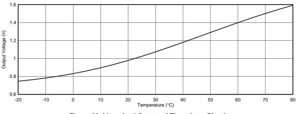
Figure 22. Linearized Output of Thermistor Circuit
