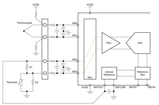
Figure 19. Thermocouple Measurement Circuit With Thermistor Cold-Junction Compensation
