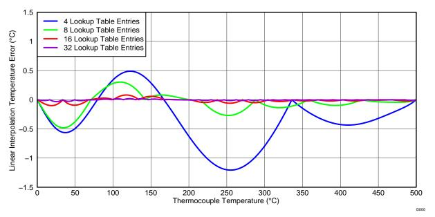
Figure 8. Comparison of Interpolation Errors Using Various Lookup Tables
