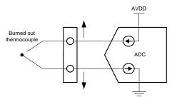
Figure 10. Burn-out Detection Using BOCS
