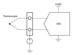
Figure 6. Voltage Biasing of a Thermocouple
