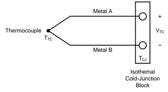
Figure 1. Thermocouple Voltage
