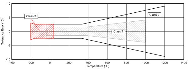
Figure 4. Type-K IEC-EN 60584-2 Tolerance Class Errors
