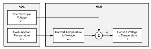
Figure 7. Thermocouple and Cold-Junction Measurement Conversion to Temperature
